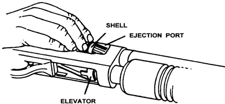
**Fig. 5 -- Loading through the ejection port**
