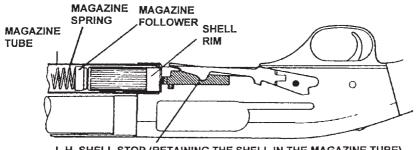
L.H. SHELL STOP (RETAINING THE SHELL IN THE MAGAZINE TUBE)
