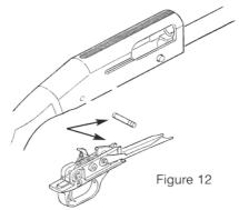
The trigger housing assembly is a complex assembly and must not be disassembled. Disassembly should only be performed at an authorized Product Service Center or by a qualified gunsmith.
