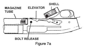
Push the shotshell into the loading port, depressing the elevator as shown in Figure 7b. This will expose the magazine tube opening within the receiver.
