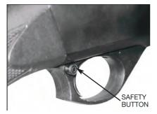
PUSH IN FULLY TO THE RIGHT UNTIL THE BUTTON MOVES NO FURTHER TO BE IN THE "ON" (SAFE) POSITION.
